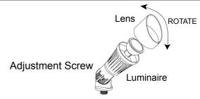
Place the lens back onto the fixture. Align the holes on both of them . Hand tighten until snug.
