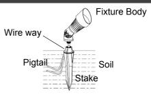
Clear away an area in the ground at the wire way on top of the stake. Lay the luminaire pigtail into the wire way and attach the luminaire onto the stake. Tighten until snug.
