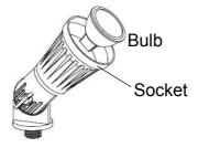
Insert the bulb with the correct wattage and type marked on the luminaire label.
