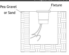
Install the fixture in the hole and fill the extra space with pea gravel or sand for proper water drainage.
