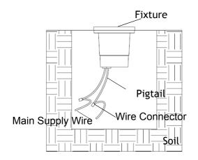
Strip both leads from the luminaire pigtail. Using two wire connectors (sold separately), connect the leads from the luminaire to main supply cable leads.
