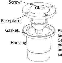
Place the grass, gasket, and faceplate back onto the housing. Secure them with the screws previously removed. Hand tighten until snug, then use a screwdriver to secure the screws using a pattern.
