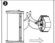
3. Connect the wires, attach the backplate, and tighten the nuts.
