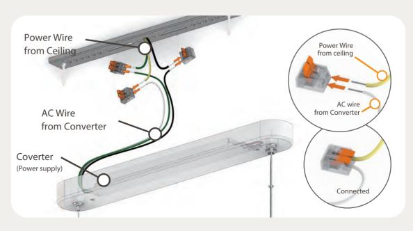
Connect converter and ceiling wiring
