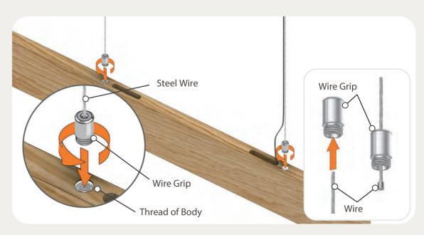
To assemble the wire to the body
