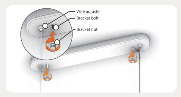
Fixing Ceiling Plate (bracket cover)
